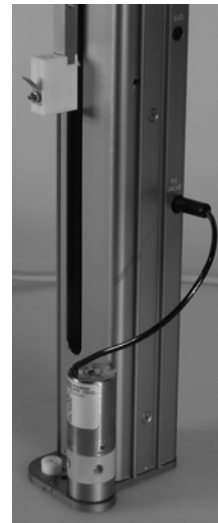
FC valve installed on the guide foot
