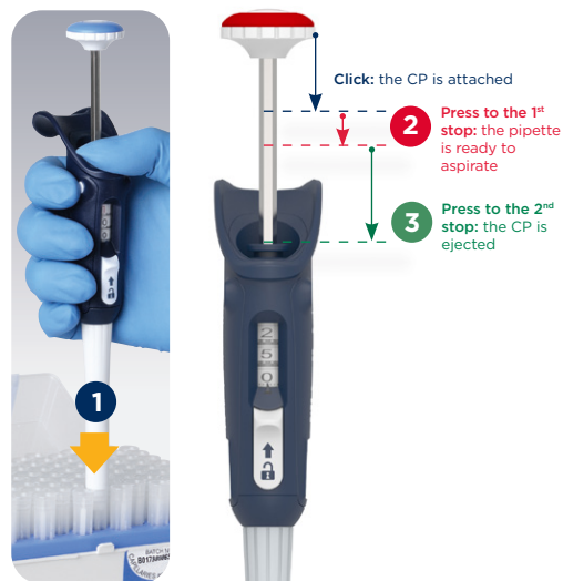
Figure 8 CP fitting on MICROMAN® E
