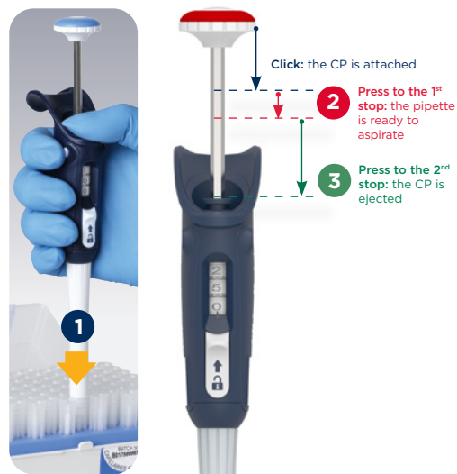
Figure 8 CP fitting on MICROMAN® E
